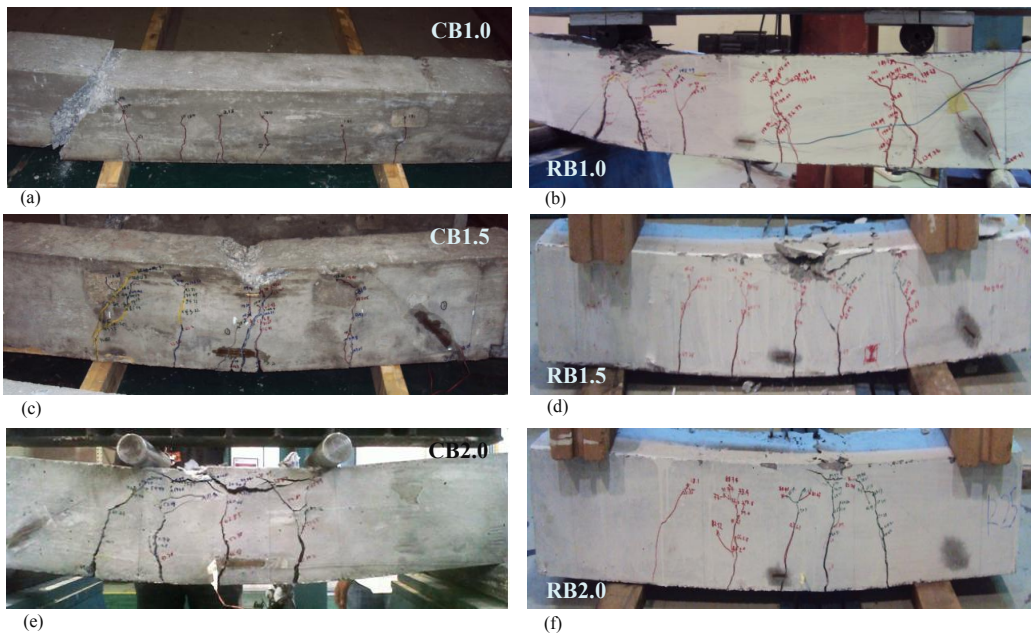
Fig.4: Crack patterns of beam specimens
